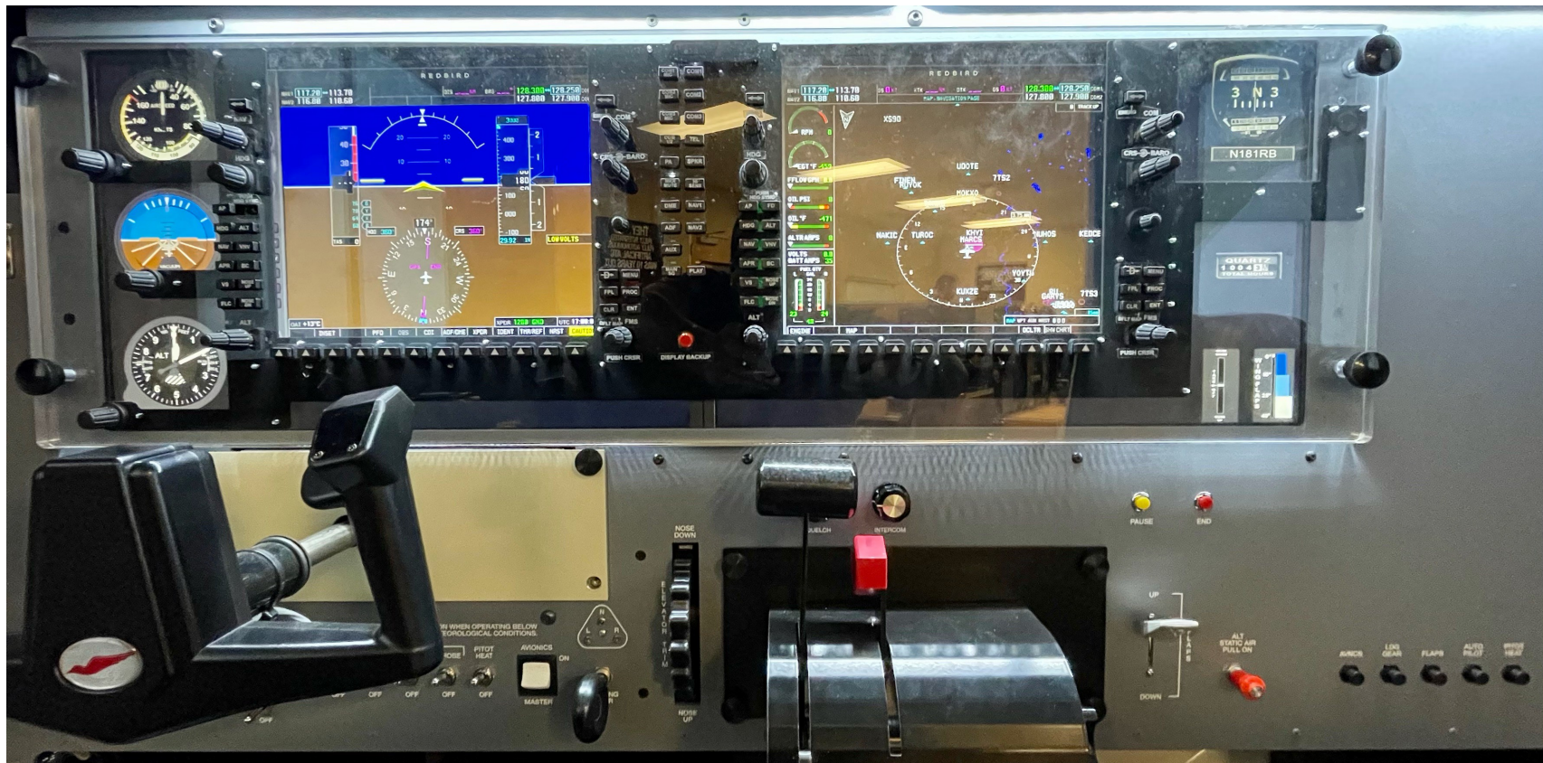
Image 11: Glass Panel Instrument Configuration (Example with Center Yoke and T-M Lever Throttle)
