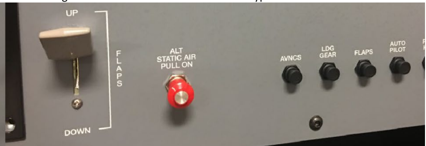
Image 29: Right Side of Lower Switch Panel Type 1, 2, & 3*
