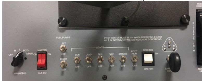
Image 26: Left Side of Lower Switch Panel Type 1 & Manual Trim Wheel*
