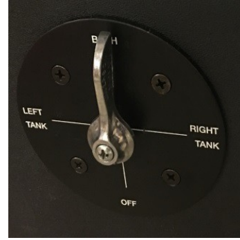
Image 42: Switch Panel 1 Fuel Selector
