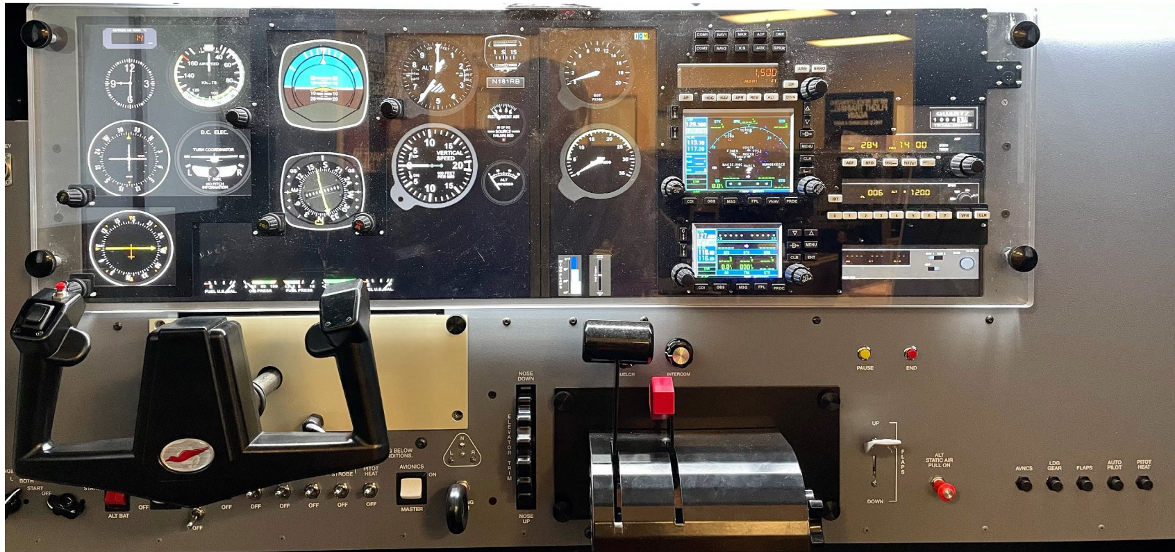
Image 10: Traditional 6-pack Instrument Panel Configuration (Example with Center Yoke and T-M Lever Throttle)
